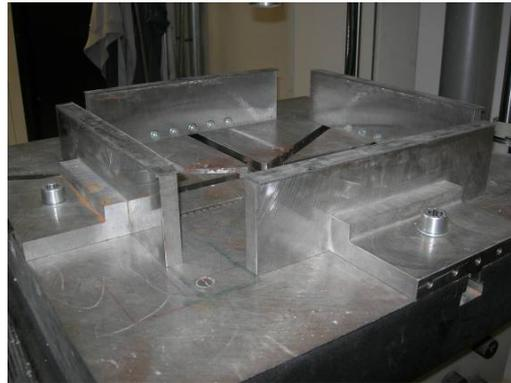
*Figure 2: Support for EN14488-5 test*
